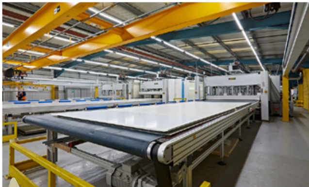
'SMART' GRP sidewall during the production process.
